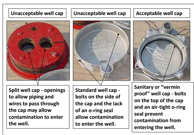
Figure 2: Photos of acceptable and unacceptable well caps
