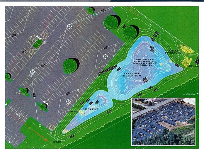
This park and ride facility was completed for use by the University of Rochester medical staff. The project included full site plan design services, agency approvals, New York State Department of Transportation turn lane addition for Scottsville Road, stormwater inspections, final pavement construction observation, and construction administration. The facility includes 600 parking spaces, bus loading areas, landscaping, lighting, and safety measures.
